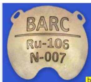
Figure 6: Different configurations of ^{106}\text{Ru} plaques: (a) Round and (b) Notched
